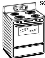
**Ranges and Ovens:** Always look inside prior to operating. Look for cracked glass and deteriorated gaskets and any obvious damage. The upper and lower burners or elements are activated to check for adequate power.
